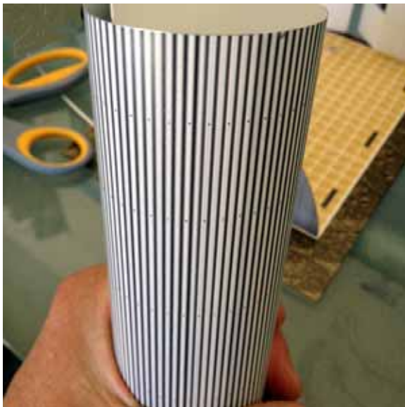
Figure 9 - Roll the roof material to pre-form it.
