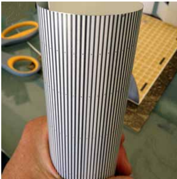
Figure 9 - Roll the roof material to pre-form it.
