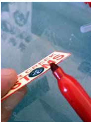
Detail edges on signs
