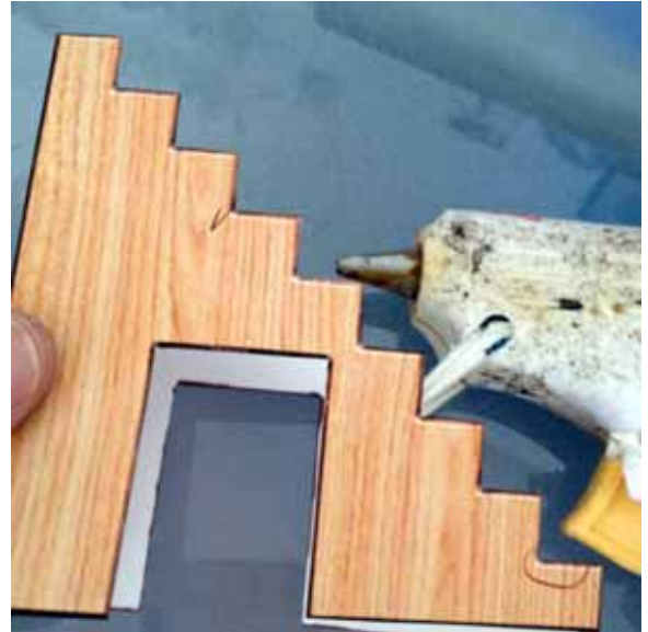
Figure 10 - Assemble the left and right center supports.
