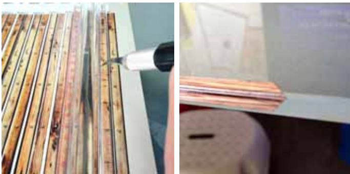
Figure 1-A, 1-B - Score the component pieces as required and fold them along the sharp edge of a table.
