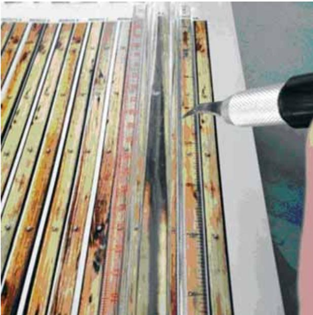
Figure 1 - Scoring the material.
